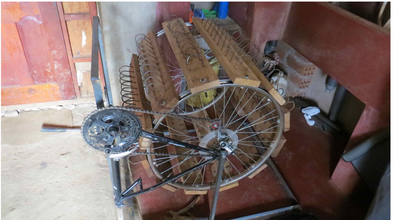
Figure 4.10: Thresher with crank arm shortened to 2 inches in length. Note the support bar above the sprockets to the left.
