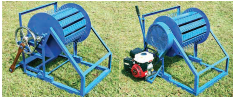
Figure 3.1 Flexible rice thresher configurations. Left, a treadle-driven design. Right, the same model adapted for motor power. Courtesy: EMBRAPA
