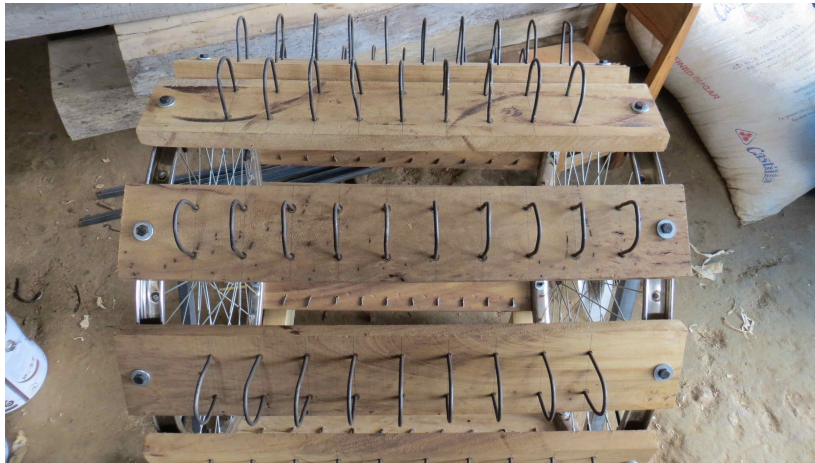
Figure 4.4: Fully assembled drum demonstrating the offset of teeth of every other plank.
