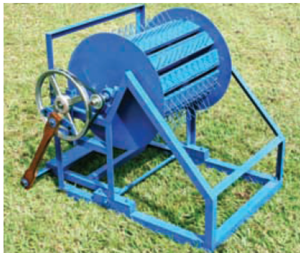
Figure 4.2: Wood and metal thresher. Courtesy: EMBRAPA
