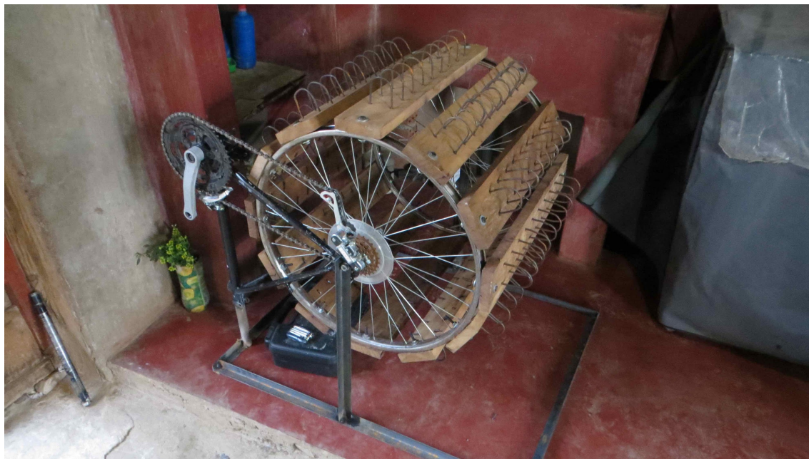
Figure 4.9: The drum seated into the frame. Note to the left the extension of the seat post so that it could stand normal to the ground. The bearings of the bicycle wheels bolt into holes in the vertical member on either side.
