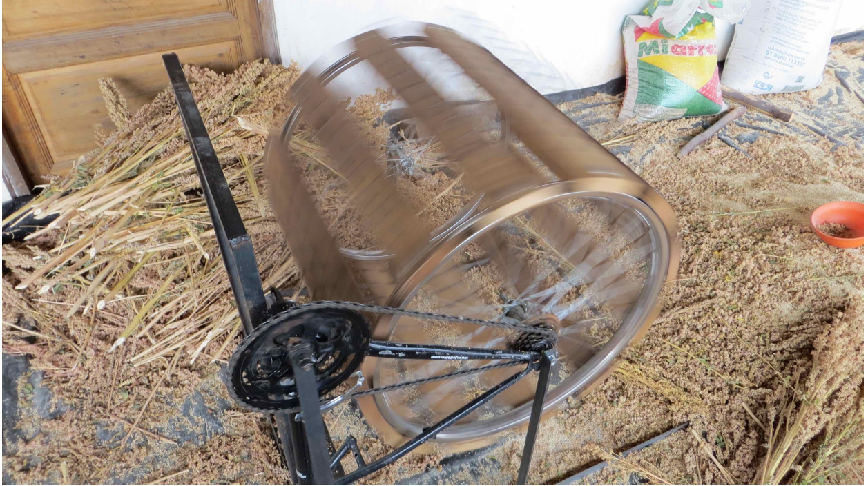
Figure 4.11: Demonstrating the functionality of the completed prototype. To the left, quinoa stacked, ready for threshing. To the right, scattered debris on the threshing floor.
